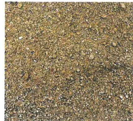
Decomposed Granite - KRC Rock 'Desert Gold' Stabilized.
